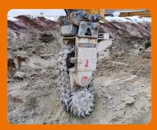
The chain cutter in close up; a chain with tungsten carbide tipped cutters runs between the cutter drums, removing the ridge of rock that normally would be left.
