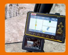
Technicians from KEMROC trading partner Beutlhauser installed a GPS control system in the excavator cab. This helped the operator excavate trenches to centimetre tolerances.
