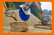
A KEMROC ES 110 HD universal cutter (110 kW) with cutter wheel (1,000 mm cutting depth) mounted on a 24-ton excavator at Fark Naturstein in the Münster region of Germany.
