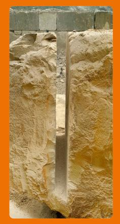
Cutting produces blocks with smooth surfaces at right angles. This makes them easier to store in the quarry and they are ideal shape for processing on the saw bench.
