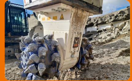
The KEMROC KRD 165 rotary drum cutter attachment in close-up. Its distinctive features include a short and compact design as well as the direct drive.
