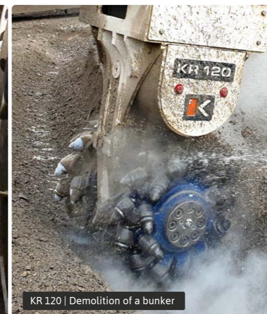
Housing with hydraulic hose protection.
