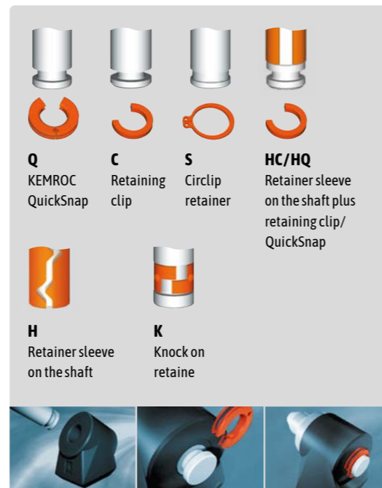
Easier and quicker pick changes with KEMROC QuickSnap.
